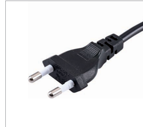
ZJ-01 2.5A 250V~ H03VVH 2 -F 2 x 0.5~0.75mm 2 H03VV-F 2 x 0.5~0.75mm 2 H05VVH 2 -F 2 x 0.75mm 2 H05VV-F 2 x 0.75mm 2
