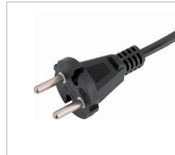
ZJ-02 16A 250V~ H05VVH 2 -F 2 x 0.75~1.0mm 2 H05VV-F 2 x 0.75~1.0~1.5mm 2 H05RR-F 2 x 0.75~1.0mm 2 H05RN-F 2 x 0.75~1.0mm 2 H05V 2 V 2 -F 2 x 0.75~1.0~1.5mm 2 H07RN-F 2 x 1.0~1.5mm 2
